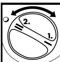
To change from one gear to the other, turn the gear selection lever through 180°.
